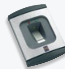
Fingerscan FL 12/FL 100 FL 12: • Up to 12 fingerprints can be taught in • Setting / programming via DIL switches on the interior device • Impulse duration: 0.5 s or 5 s FL 100: • Up to 100 fingerprints can be taught in • Setting / programming via 3 buttons and two 7-segment displays on the interior device • Impulse duration: programmable from 0.5 s – 90 s
