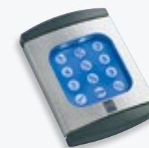
Code switch CTR 1b/3b CTR 1b: 1 relay output for control of one door operator CTR 3b: 3 separate relay outputs for the control of 2 operators and/or choosing the direction, second opening height, yard illumination, Stop
